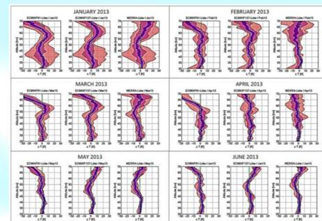
Distribution of the monthly difference between ECMWF (L91 and L137) and MERRA (Modern-ERA Retrospective Analysis for Research and Applications) temperature models at 0h UTC and nightly averaged lidar measurements versus altitude at OHP from January to June 2013.
