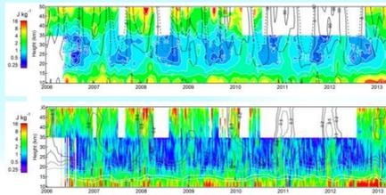
Combined time series of GW Ep from Rayleigh lidar at OHP and COSMIC GPS Radio Occultation data (5° x 5° domain centered at OHP). a) Monthly-mean Ep (color map) and zonal wind (solid contours - westerly winds of 30 and 80 m/s, dotted contour - zero wind, dashed contour - easterly wind of 10 m/s). b) Weekly means of Ep from COSMIC and lidar (color map) and monthly means of MERRA Ep (Khaykin et al., 2015).
