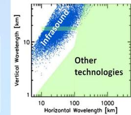
Thirteen years of gravity wave activity measured at IS17 infrasound station (Ivory Coast). The color scale indicates the logarithm of the number of detections. The seasonal variations of the wave azimuth are related to thunderstorms and to the tropical rain belt partly related to the Intertropical Convergence Zone of the winds (Blanc et al., 2014).
