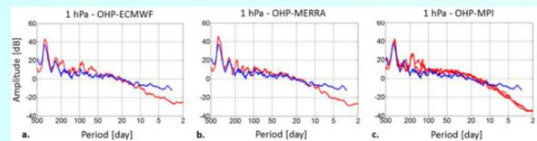
Comparison between lidar (blue) and model (red) periodograms at 1 hPa (~47 km) over OHP. (a): ECMWF (2003-2013). (b): MERRA (2003-2013). (c): MPI-ESM-LR (1991-2005), each line corresponds to one ensemble member (Le Pichon et al., 2015).
